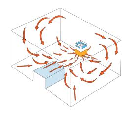
This slow moving flow occurs for the entire room, including corners. Surface depositing is significantly reduced.
