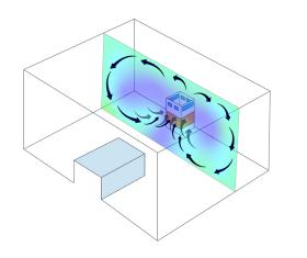
The rotational flow forms a rotational motion, within the slow moving whole room air system.
