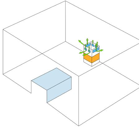
Ultra Clean Air, near sterile, exits the system and rotates upwards to form a return path.
