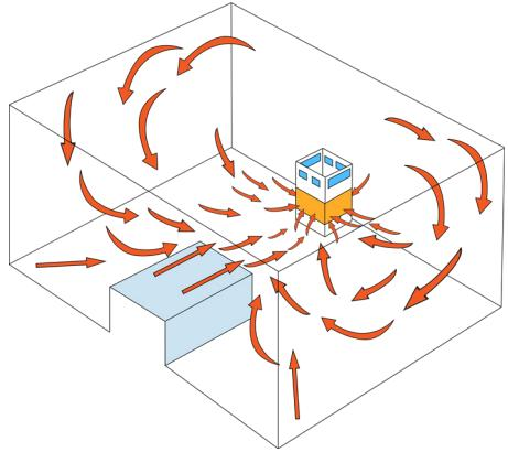
This slow moving flow occurs for the entire room, including corners. Surface depositing is significantly reduced.
