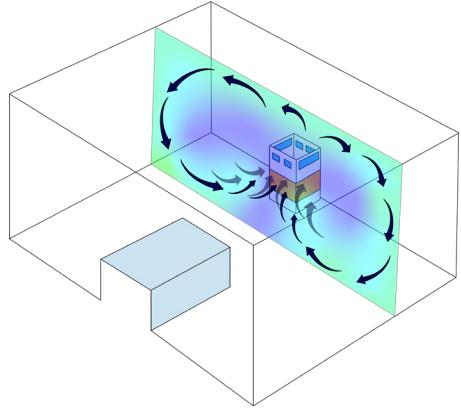
The rotational flow forms a rotational motion, within the slow moving whole room air system.
